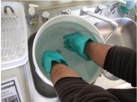
Place un-preserved sample vial under water and remove cap. Hold tubing and allow flow into vial and displace two vial volumes.
