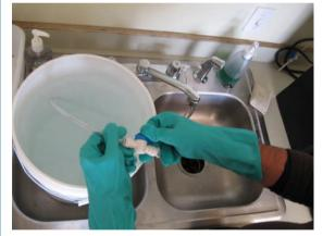
Remove aerator. Attach apparatus to faucet feed tubing to a clean 5 gallon bucket and fill to the top.
