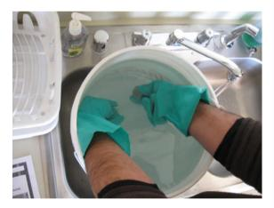
Make sure vial is at the bottom of the bucket and replace cap to trap any dissolved methane.
